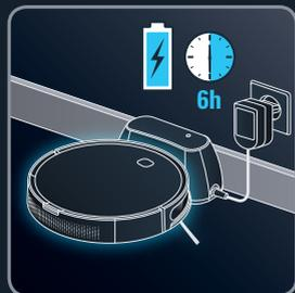
**EN** Wait 6 hours for the robot to be fully charged.
